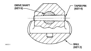
Figure 21. Taper Pin Installation for Fisher V150, V200, and V300 NPS 1 Valves with Micro-Notch Ball Construction
