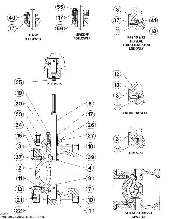
Figure 25. Exploded View, Fisher V150 and V300 (NPS 3 - 12) and Flanged V200 (NPS 3-8) without Attenuator Assembly.
