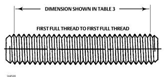
Table 3. Flange Stud Lengths Required for Seal Protector Ring End of Fisher V150, V200, and V300 Valves
