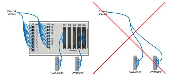
Use of several safety modules with a terminal adapter implies to have a consistent configuration between the connected safety modules. For example, but not limited to, a consistency between the configuration of the inputs and outputs of each safety module.
