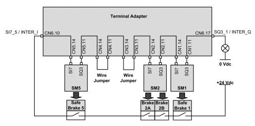
Both [SQ3 function assignment] 5 *L* / 2 and [SI7 function assignment] 5 *L* / 3 of each chained safety module are set to SBC Feedback.
