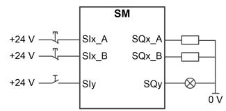
Six\_A and Six\_B: Safety Input x (Channel A and B) Siy: Safety Input y SQx\_A and SQx\_B: Safety Output x (Channel A and B) SQy: Safety Output y
