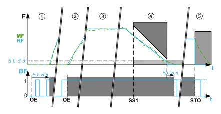
F: Frequency / MF: Motor Frequency / RF: Reference Frequency
