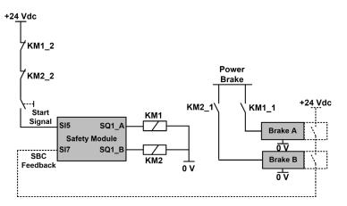
SBC feedback signal (dotted line) is an optional signal. The wiring of KM1\_2 (or KM2\_2) contact on the start signal helps to prevent the start of the safety module in case of welding contacts on the relay KM1 (or KM2) if KM1\_2 and KM1\_1 (or KM2\_2 and KM2\_1) are mechanically linked.
