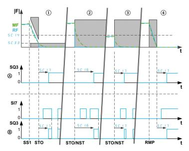
**|F|**: Frequency (Absolute value) / **RF**: Reference Frequency / **MF**: Motor Frequency **t**: time
