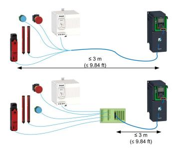
Verify that the wiring, cables, and connected interface meet the PELV (Protective Extra Low Voltage) requirements.
