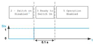
SIX Inputs assigned to the safety function SS1
