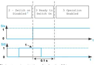
SIx Inputs assigned to the safety function SS1
