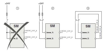
There are three ways of connecting the signals to the safety module
