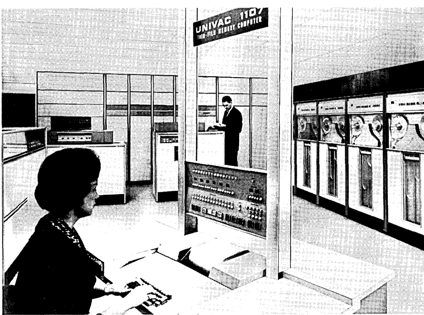
UNIVAC 1107 THIN-FILM MEMORY COMPUTER UNIVAC Division, Sperry Rand Corp. New York, N.Y.
