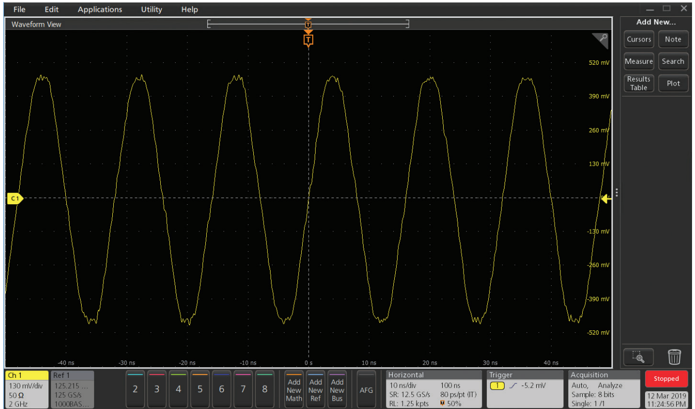
Figure 3. Test Mode 2 for 1000BASE-T alternates between +2 and -2.
