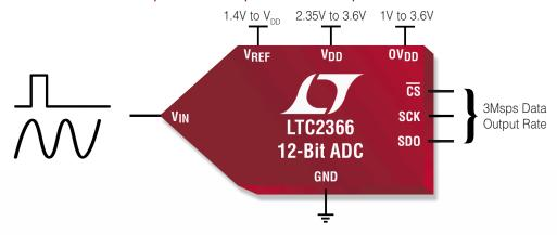
The LTC®2366 family of SAR ADCs offers sampling rates from 100ksps to 3Msps in pin-compatible 6- and 8-lead SOT-23 packages. With high impedance, single-ended analog inputs and the ability to operate with reduced spans, these ADCs can connect directly to sensors and transducers without the need for gain stages. The high sample-rate-to-power ratio makes these ADCs ideal for compact, low power, high speed systems.
