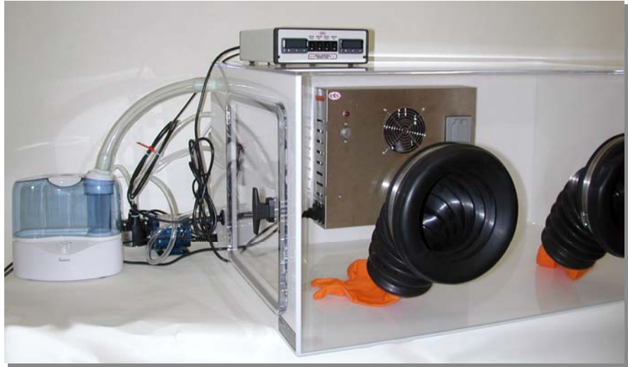
Figure 1.2-2: Package B Humidity and Heating Control System
