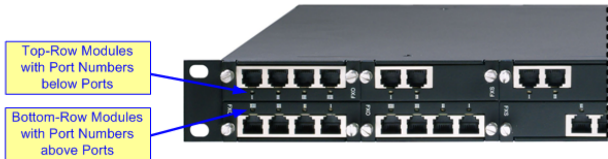
Figure 6-3: Module Orientation in Chassis Top- and Bottom-Row Slots
