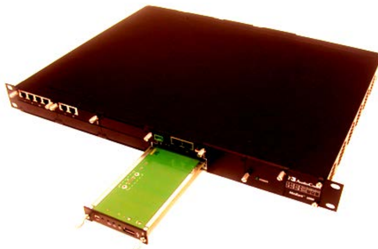
Figure A-5: Inserting CM Module in Front-Panel Slot
