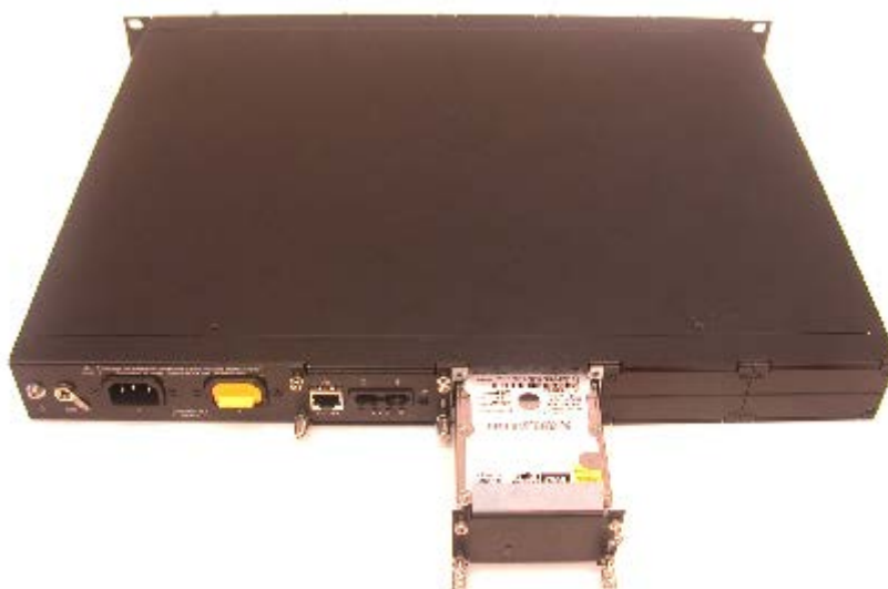
Figure A-9: Inserting HDMX Module in Rear-Panel Slot
