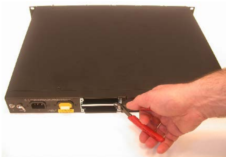
Figure A-7: Cutting Metal Strip
