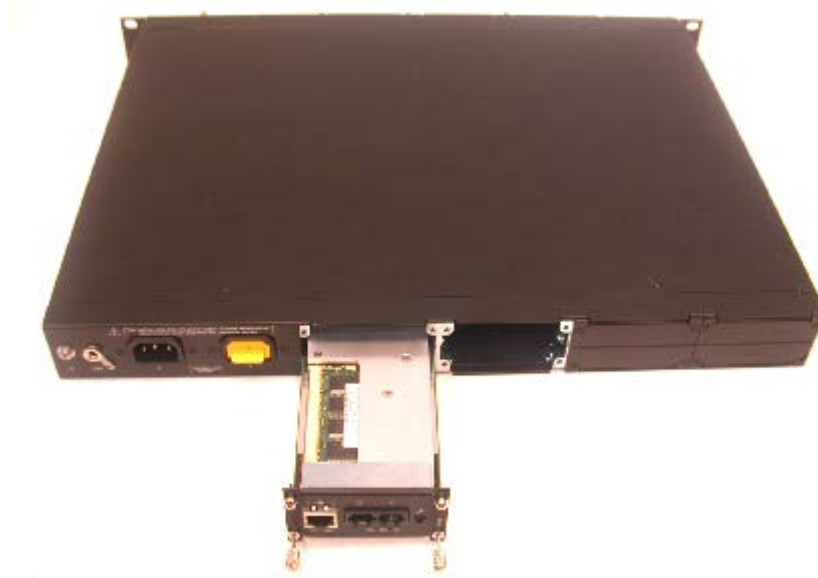
Figure A-8: Inserting iPMX Module in Rear-Panel Slot
