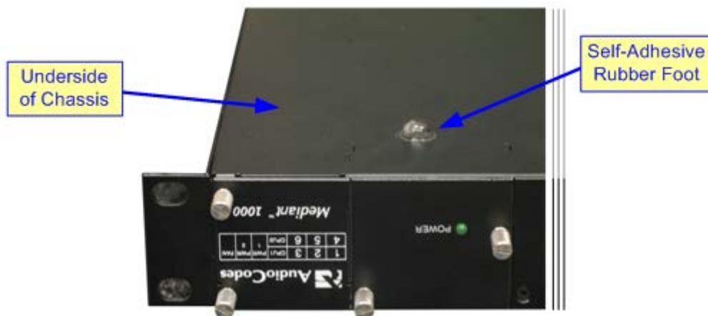
Figure 4-1: Attached Rubber Bumpers on Underside of Chassis
