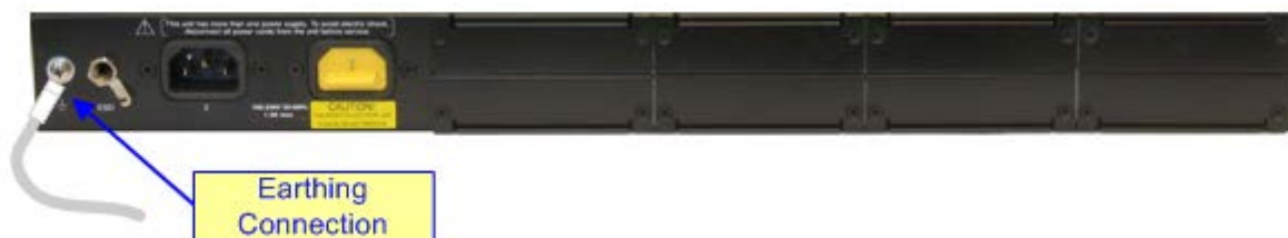
Figure 5-1: Grounding the Device
