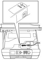
Carefully guide the USB cable into the cable channel and out the back of the machine. Connect the cable to your Macintosh.
