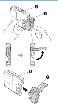
Take care to match the sticker colour ① with the cartridge colour ② as shown in the diagram below.
