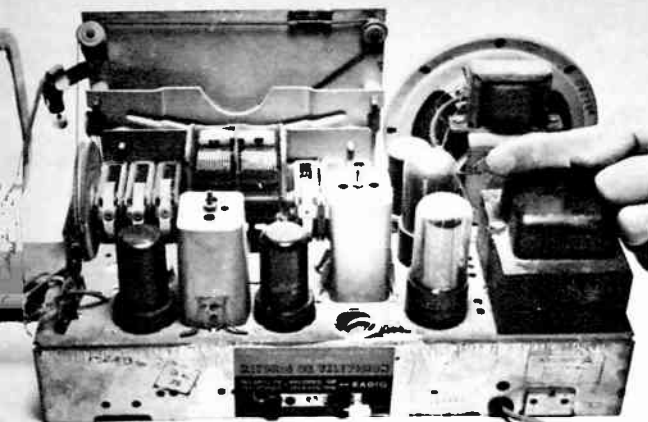
Left: Neglected chassis is thick with dust, encrusted with kitchen grease, and a home for insects. Dust is especially bad because it prevents proper radiation of heat from hot tubes, other components.
