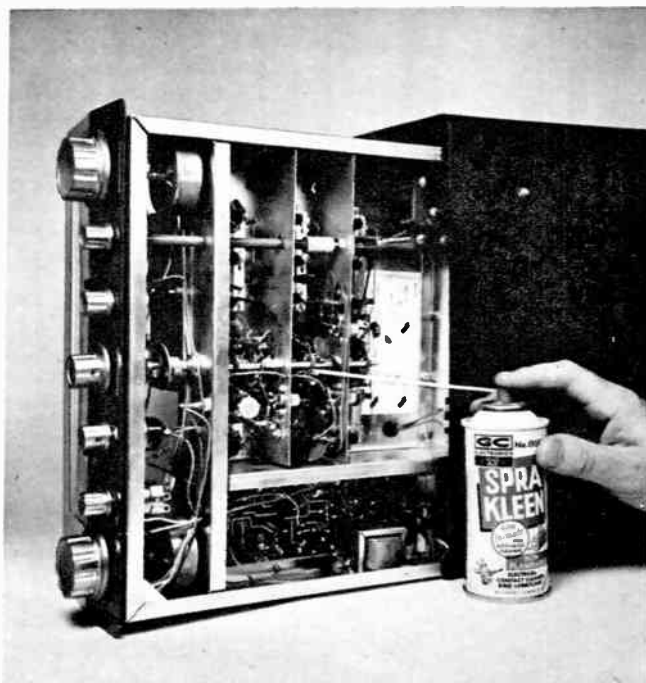
Above: Five-band "Mohican" receiver, made from a Heathkit, is a solid-state set. Works either on dry cells or AC power unit. The slide-rule dial has separate scales for regular tuning of AM and short-wave bands and for band-spreading the special ham bands.
