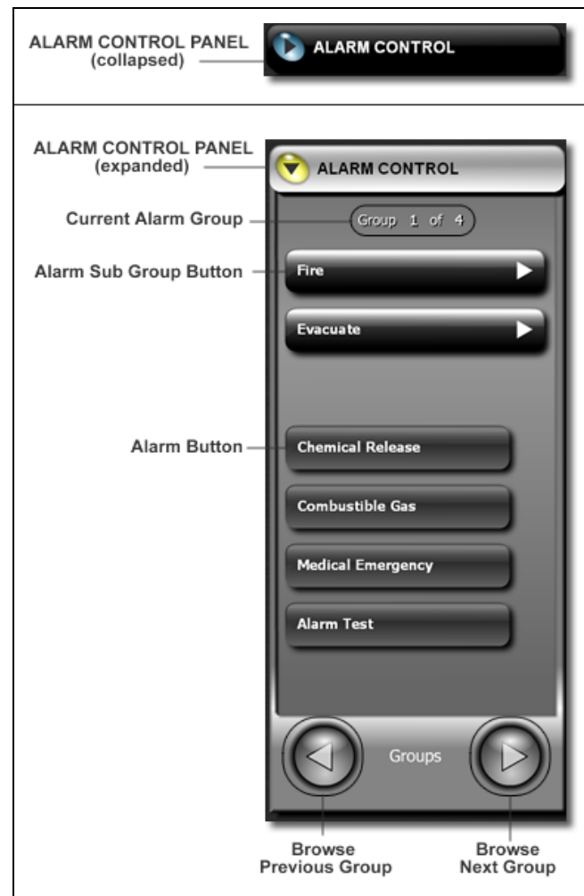
Figure 14. Alarm Control Panel
