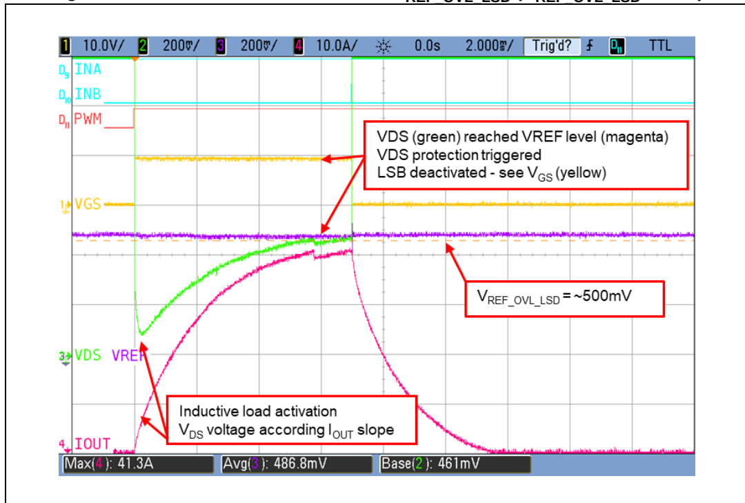
Figure 21. Load activation with too low V_{REF\_OVL\_LSD} ( R_{REF\_OVL\_LSD} = 10\text{ k} )
