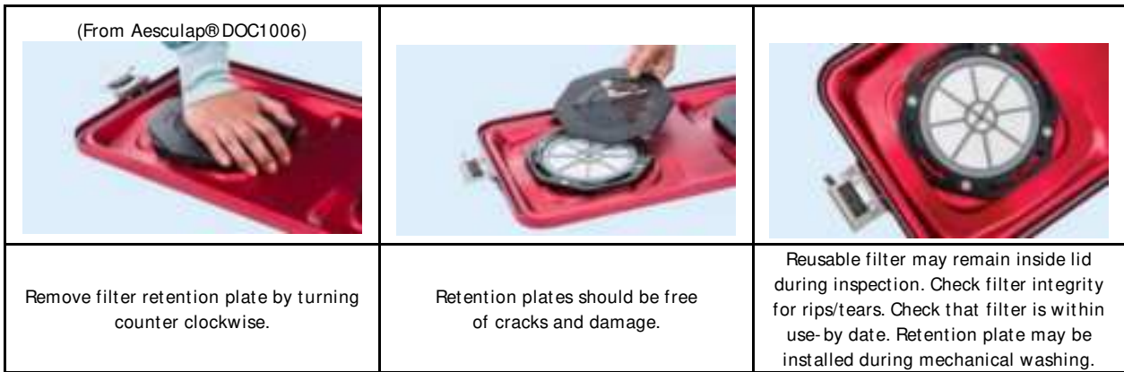
Image 4: PrimeLine™ Lid Inspection Process
