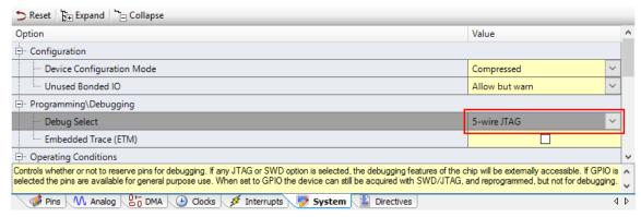
When either SWD (default) or GPIO is selected in this option, JTAG pins are disabled in the user application start-up code. This causes PSoC Programmer or 3rd party tools to be unable to access the device using JTAG protocol.
