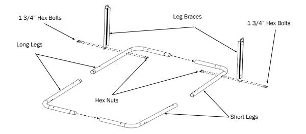
**Step 2:** Install Bottom Wire Shelf by placing the four corner hooks inside the hole on each leg then rotate the leg assemblies up and secure the Leg Braces to the other side of the Long Leg and Short Leg set.
