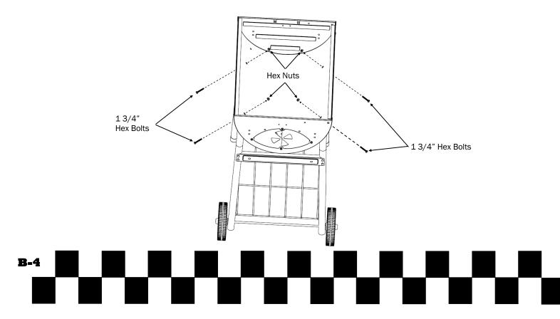
**Step 5:** Attach Damper Circle to the side of the Grill Body with one Hex Bolts, two Flat Washers, one Lock Washer, and one Hex Nut.
