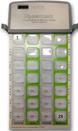
Figure 5: Smart Connector with Printed Foil Blister Pack
