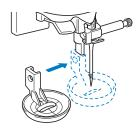
Tighten the screw with the included screwdriver.
