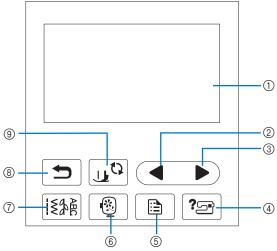
1) LCD (liquid crystal display) (touch panel)
