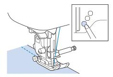
Press (Thread cutter button) to trim the upper and lower threads.
