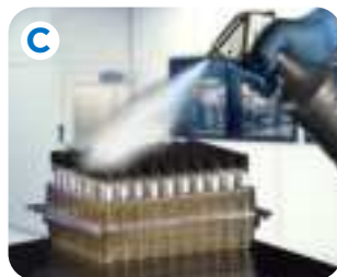
C Spray down entire ReadyRack™ with isopropyl alcohol.
