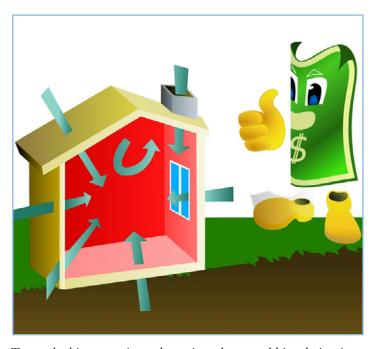
To get the biggest savings, the easiest place to add insulation is usually in the attic. A quick way to see if you need more insulation is to look across your uncovered attic floor. If your insulation is level with or below the attic floor joists, you probably need to add more. The recommended insulation level for most attics is R-40 (or about 12 to 15 inches, depending on the insulation type). In the coldest climates, insulating up to R-50 is recommended.
