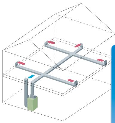
leaks using mastic sealant or metal (foil) tape and insulating all the ducts that you can access such as those in the attic, crawlspace, basement, or garage. Do not use "duct tape," as it is not long-lasting.
