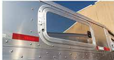
Sealed Access Door on Side
