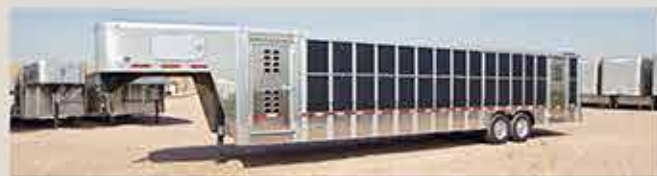
Extruded Aluminum Post Side Construction with Cold Weather Panels
