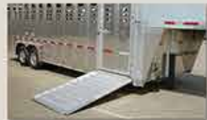
Side Loading Ramp
