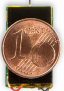
Fig. 3: The ICARUS tag (a virtually series-ready prototype is shown here in actual size) was developed jointly by the Max Planck Institute for Ornithology and I-GOS. It is an autonomously operating multi-sensor device with a radio module (see the overview box on the left for the sensors). The tag communicates with the ISS and with terrestrial base stations.
