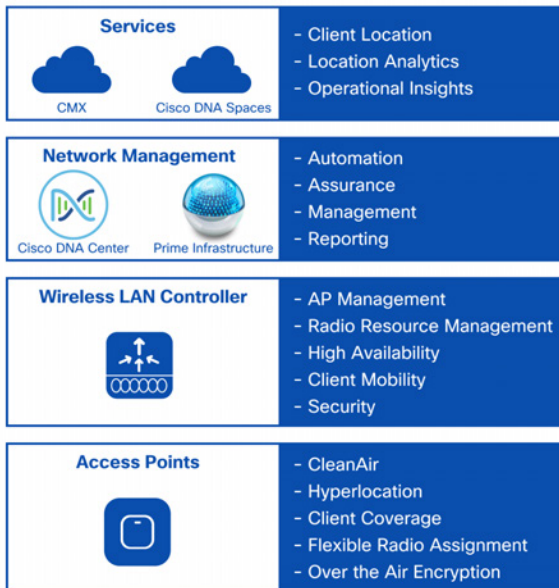
DIAGRAM Primary components of intent-based networks for wireless
