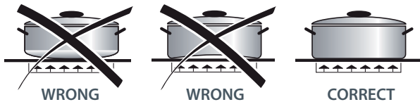
Inefficient and efficient saucepan bottoms
