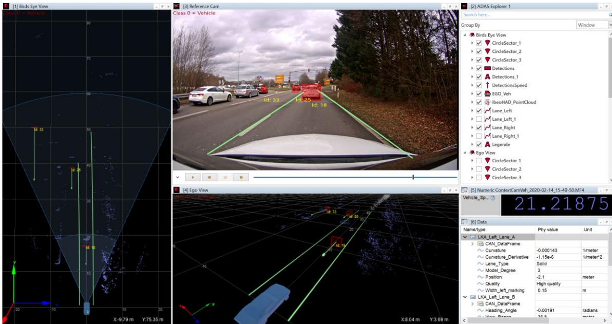
Figure 10: Option Driver Assistance – Object verification for checking algorithms in the development of driver assistance systems.
