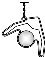
30° Mounting With “Combination” Hanger
