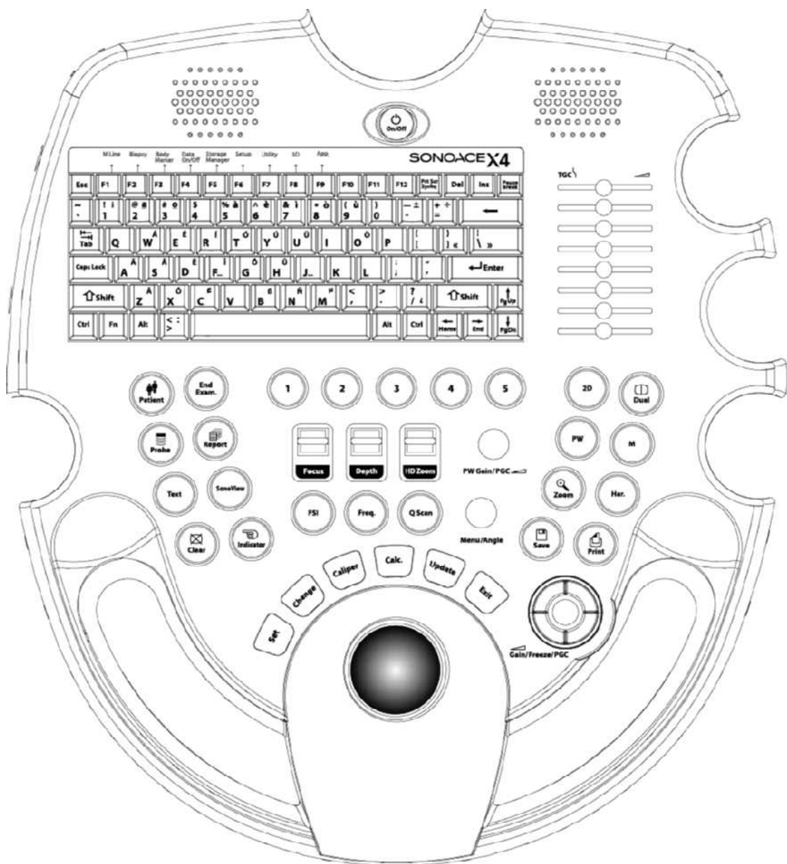
[Figure 2.8 Control Panel]
