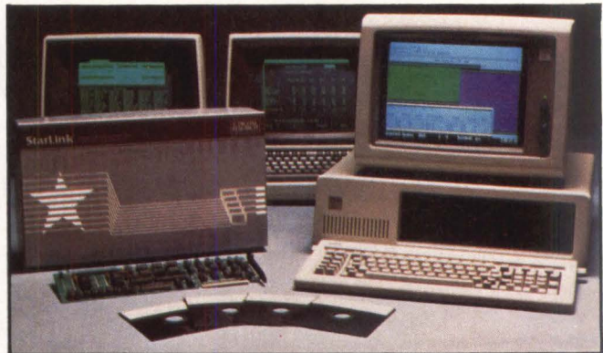
Extending the operating environment of the IBM PC can be achieved using DRI's Concurrent CP/M-86 and a Starlink expansion add-on to support as many as five users.
