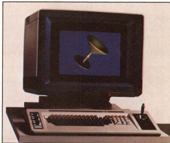
The Merlin 9200 computer-integrated-design graphics terminal combines a graphics engine with a local database and a local task processor.
