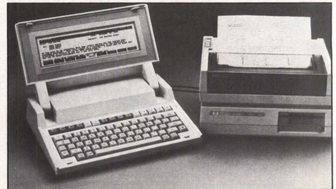
HP's Portable weighs 9 pounds, features a 16-line-by-80-character display, built-in application software like word-processing and spreadsheet programs, and terminal-emulation capabilities.
