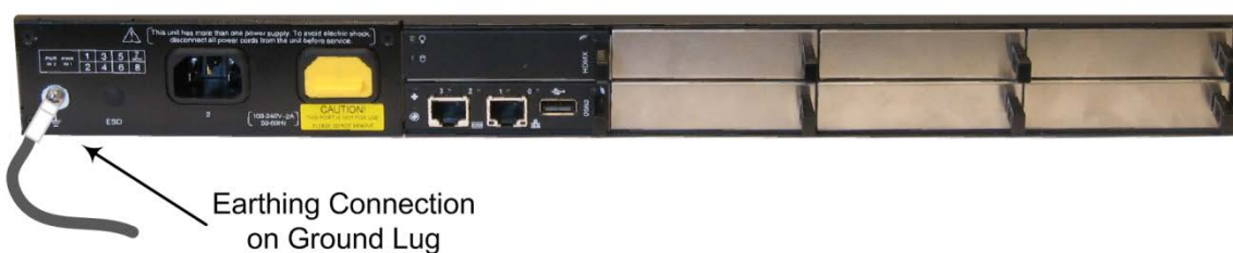
Figure 6-1: Grounding the Device
