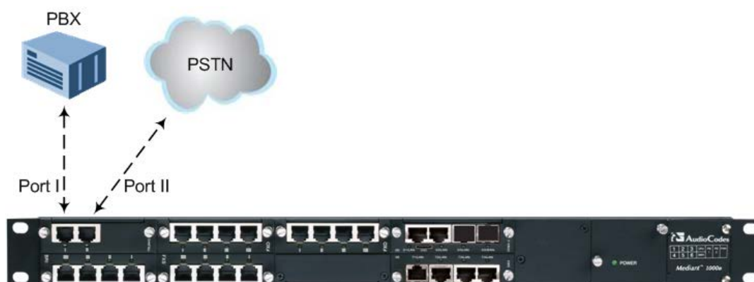
Figure 6-9: Cabling (Ports 1 and 2) PSTN Fallback
