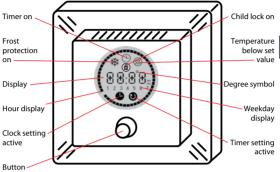
The thermostat is operated by using the button as follows:
