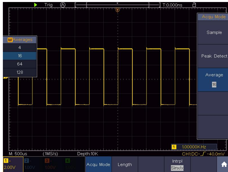
Figure 6-5 Reduce Noise level by using Average function
