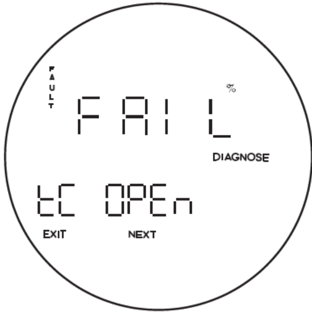
Figure 5-5. Fault 1, Open Thermocouple
