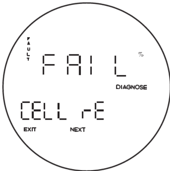
Figure 5-11. Fault 7, Reversed O 2 Cell
