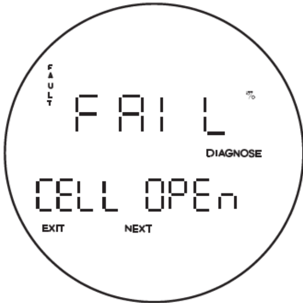
Figure 5-9. Fault 5, O2 Cell Open
