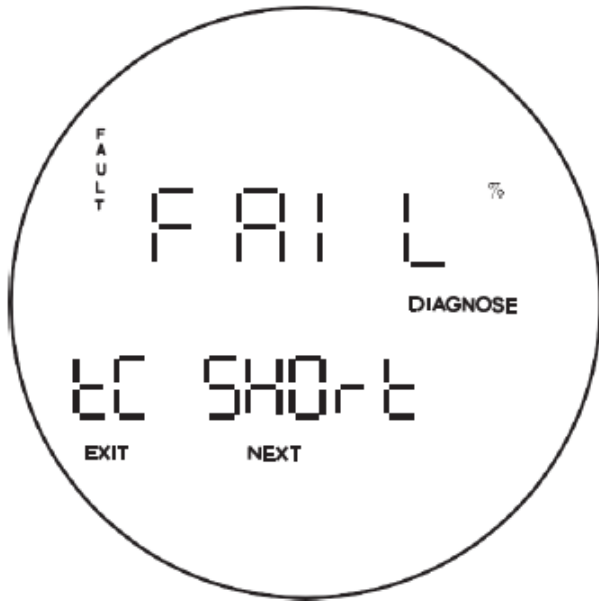
Figure 5-7. Fault 3, Shorted Thermocouple
