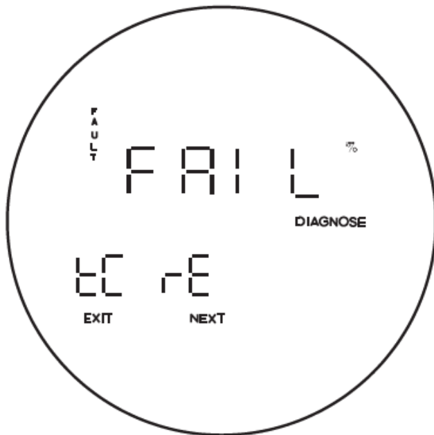
Figure 5-6. Fault 2, Reversed Thermocouple
