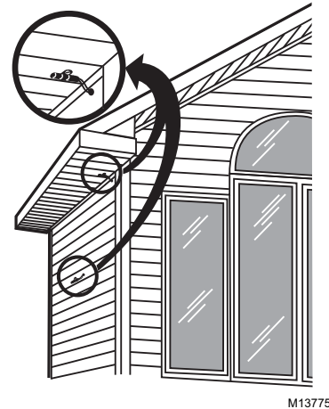
Fig. 7. Outdoor temperature sensor installation.
