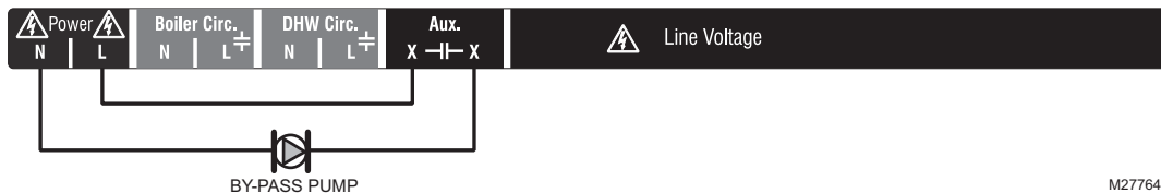
Fig. 16. Wiring of the Aux. pump line voltage rated dry contacts [example shown is for a by-pass pump].
