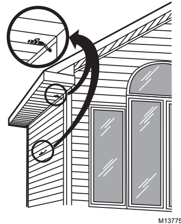
Fig. 7. Outdoor temperature sensor installation.
