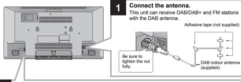
Connect the AC mains lead after all other connections are completed.
