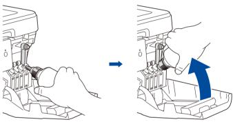
Remove the nozzle cap and insert the bottle nozzle firmly into the ink tank so that the ink does not spill.
