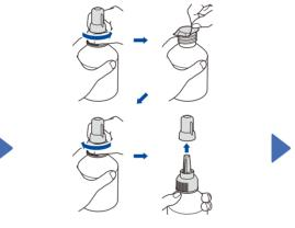
Remove the film and tighten the cap firmly.
