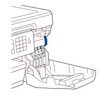
Push down on the cap of the ink tank to close it tightly. Repeat step 6 for the three other ink tanks.
