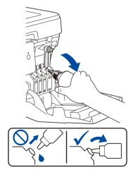
When finished, remove the bottle, pointing the nozzle upward so the ink does not spill.
