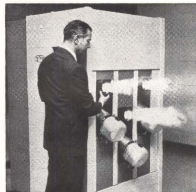
THREE black-and-white Eidophor optical units plus filters make up color-tv projection system
