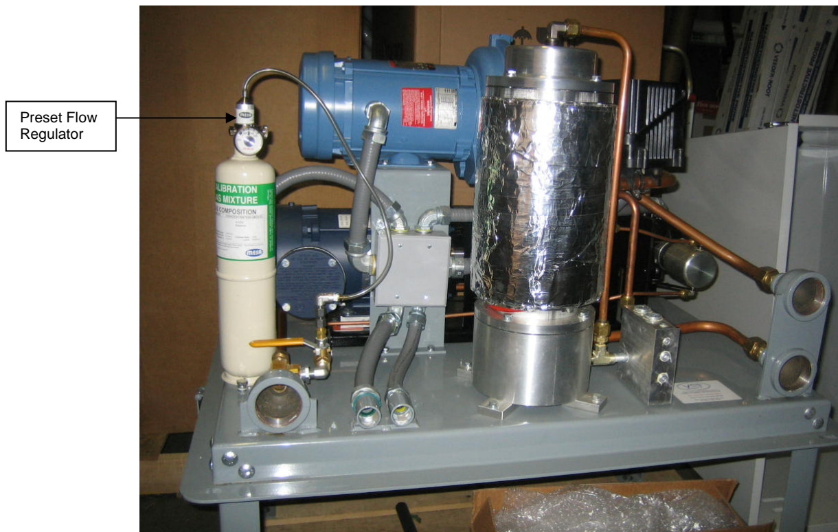
Figure 2 Equipment Configuration for Verifying Hydrocarbon Sensor Performance
