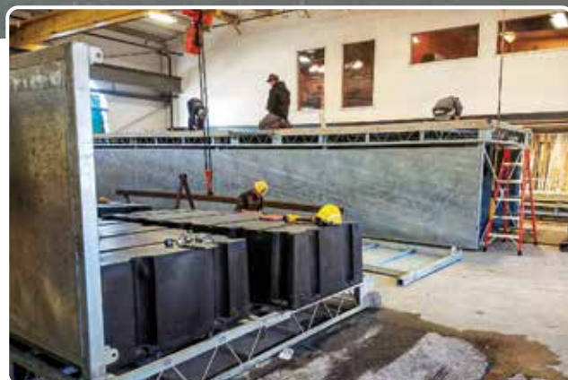
Wave attenuators during production in our manufacturing facility.
