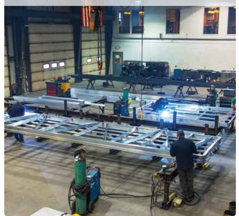
Aluminum docks being manufactured.
