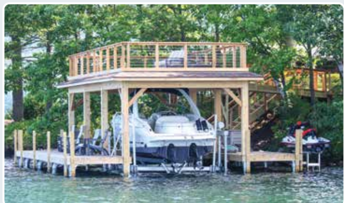
Crib dock with sundeck style boathouse and sling style boathouse lift.
