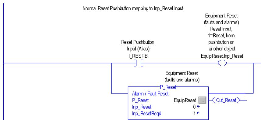
The following illustration shows EnableIn False implementation with the input condition mapped to the P\_Reset instruction by using the Rung-In state.
