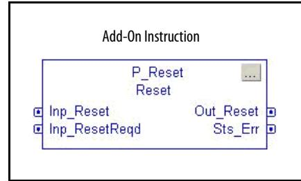
The P\_Reset instruction accepts an Operator Reset command, a Program Reset command, and a Reset Input that can come from a push button, from a higher-level P\_Reset instruction (from a containing control strategy, such as a Unit Reset sent to a P\_Reset at Equipment Module scope), or from any other source.
