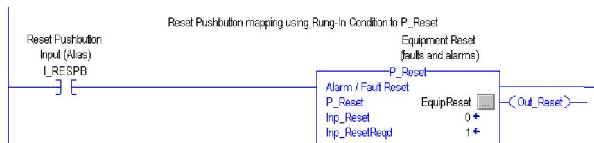
The Rung-In condition determines whether the P\_Reset instruction's normal code (Logic Routine) is performed or its EnableIn False code (EnableInFalse Routine) is performed. In the P\_Reset instruction, the EnableIn False code is identical to the Logic code, except it also arms a one-shot for the Rung-In condition. When the rung goes **True**, the Logic routine one-shot fires and the Out\_Reset output pulses for the configured time, executing a reset.
