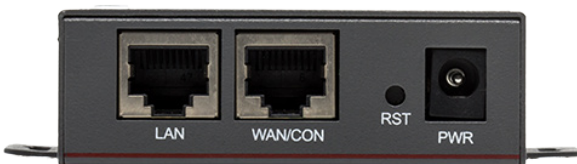
Figure 5. LAN, WAN/CON, Reset and Power Interfaces
