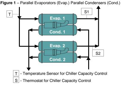
Depending on the number of units and operating characteristics of the units, loading and unloading schemes should be designed to optimize the overall efficiency of the chiller plant. It is recommended to use an evaporator bypass piping arrangement to bypass fluid around evaporator of any unit which has cycled off at reduced load conditions. It is also recommended to alternate the chiller cycling order to equalize chiller starts and run hours.
