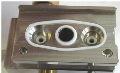
Fig. 73: Seal installed in the pump head
