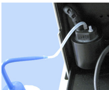
Fig. 28: Filling water into the connection port
