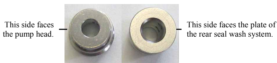
Fig. 74: Orientation of the rear seal wash body
