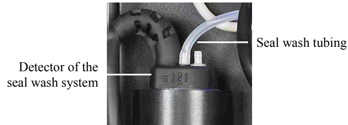
Fig. 61: Detector of the seal wash system
