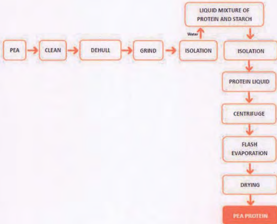
Figure 2. Manufacturing Process of Pea Protein
