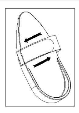
The pedal strap is adjustable and can be personalized to fit the user's foot size.
