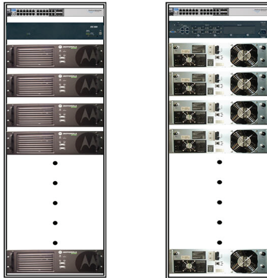
Figure 32: Rack Mounting of Components of a Single Site System.
