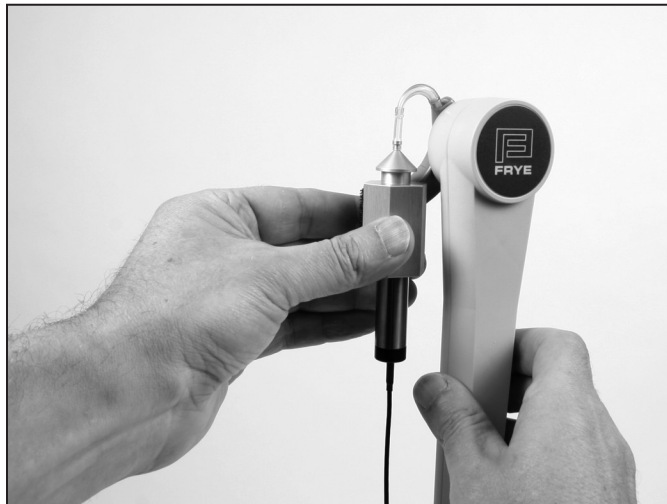
Figure 5.1.5—Holding telewand parallel to the body of a BTE
