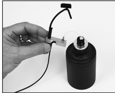
Figure C-3: Integrated probe microphone inserted into sound calibrator.
