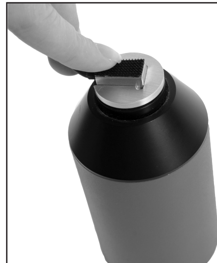
Figure C-4: Rectangular reference microphone inserted into sound calibrator.
