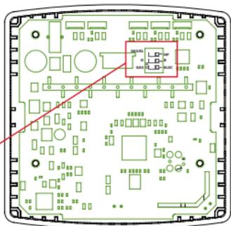
\*Reversing valve choice, 0 or B, is dependant on the type of valve installed in the heat pump.
