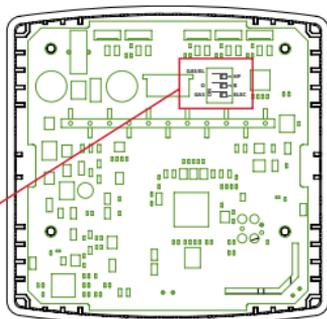
\*Reversing valve choice, O or B, is dependant on the type of valve installed in the heat pump.
