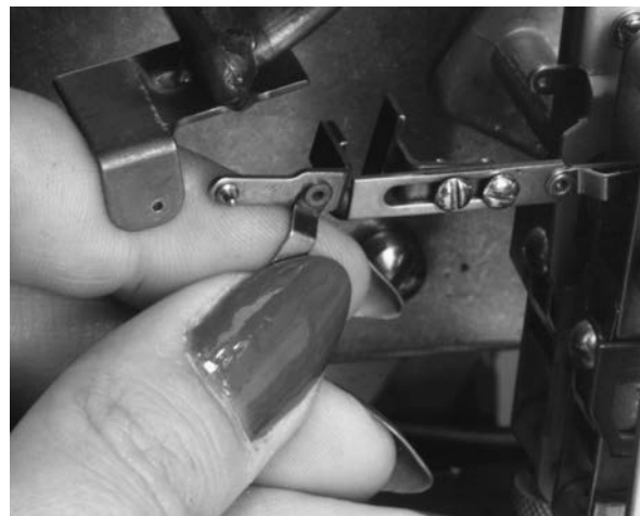
Figure 6-14. Disconnecting Link 1 from the Bourdon Tube
