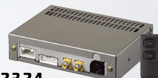
EA1232A POWER BOX FOR CJ981E • One camera direct input • Signal connection for indicator lights or reverse gear • Includes wired remote controller for Iris & Zoom settings • AUX video input (NTSC / PAL) • 12V/24V compatible
