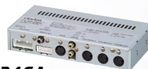
EA1246A POWER BOX FOR CJ981E • Three camera direct inputs • Three signal connections for indicator lights and reverse gear • Compatible wired remote controller for Iris & Zoom function (RCB174) • AUX video input (NTSC / PAL) • 12V/24V compatible
