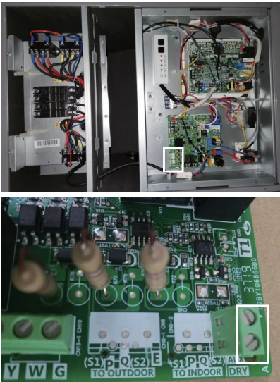
Fig. 29 — Connect the auxiliary heat wire
