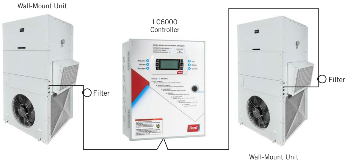
FIGURE 21 Communication Wiring (Alternate Method)
